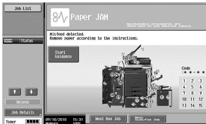
A flashing "round number" indicates the location of the paper jam/staple jam.
