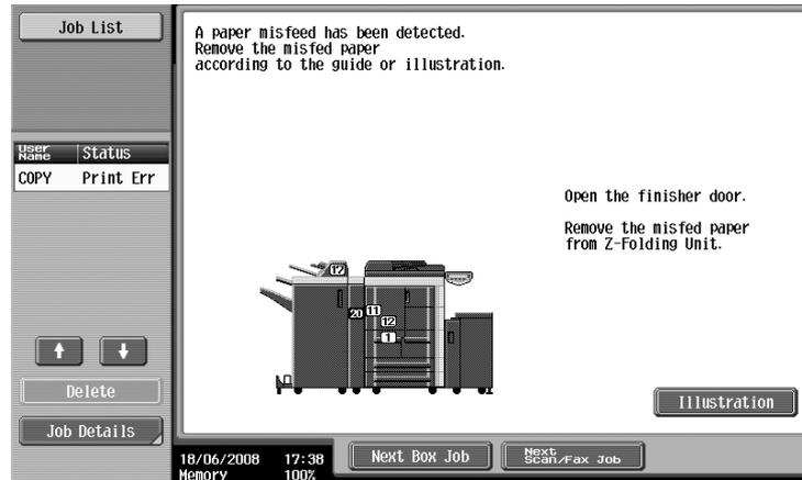
Touching the [Illustration] key on the Misfeed Location screen displays another screen with the message "Remove the misfed paper according to the guide or illustration.", and also with a description and illustration for clearing misfed paper.
