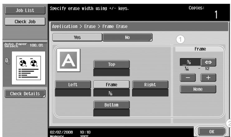
*Frame Erase: The same width can be erased on all four sides of the original, or the width that is erased can be specified for each side.
