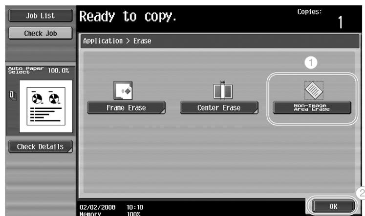
*Non-Image Area Erase: Detects the original size placed on the original glass and erases outside area of the original.*
